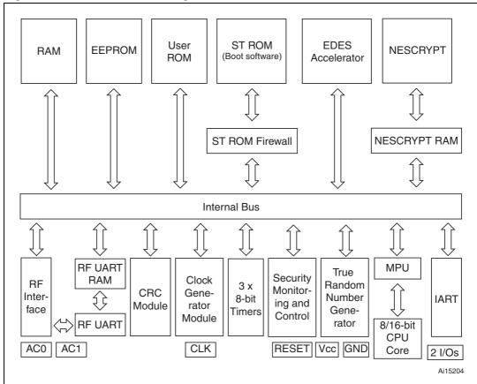
Figure 1. ST23YR04 block diagram
