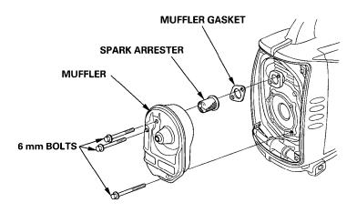
3. Use a brush to remove carbon deposits from the spark arrester screen.
