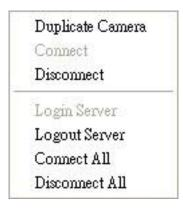
• **Duplicate Camera**: Select the duplicate camera function to create multiple views. The duplicated camera will be shown with green indicator as the right picture. Combine this function with digital PTZ, users are allowed to enlarge different spots and view them in different channels
