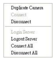
• **Duplicate Camera**: Select the duplicate camera function to create multiple views. The duplicated camera will be shown with green indicator as the right picture. Combine this function with digital PTZ, users are allowed to enlarge different spots and view them in different channels without failing to record the whole view.
