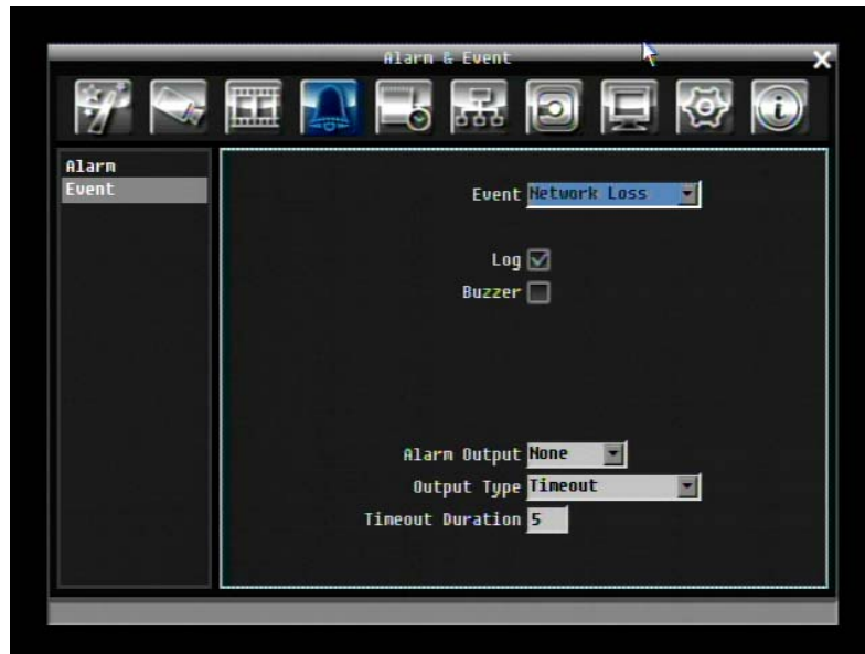
Figure 10-17 Alarm &amp; Event Menu – Event – Network Loss
